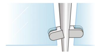
• Figure 2 Glass under stress due to misaligned clamp fixing
