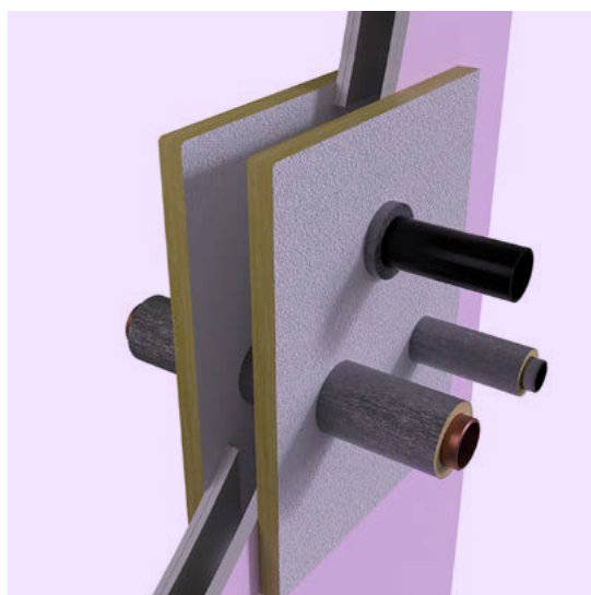
Figure 9 Unframed opening in drylining
