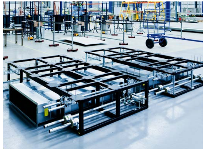
Figure 4 Example of a prefabricated corridor M&E module
