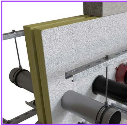
Figure 29 Support of services on either side of the compartment
