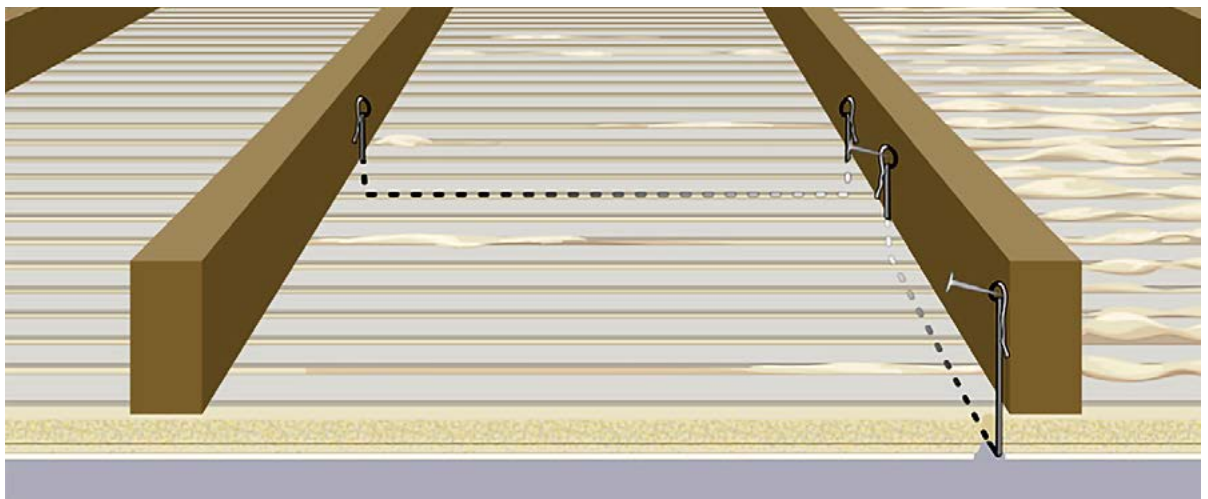
Figure 18: example wire staples.
