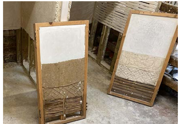
Figure 3: example boards showing earth mortars on reed (left) and lime plaster on laths (right) (Sean Wheatley).
